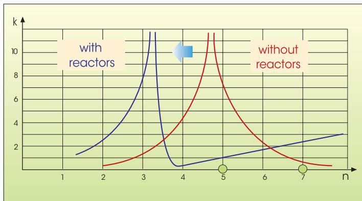
Shifting Resonance Frequency Below the 5<sup>th</sup> Harmonic
